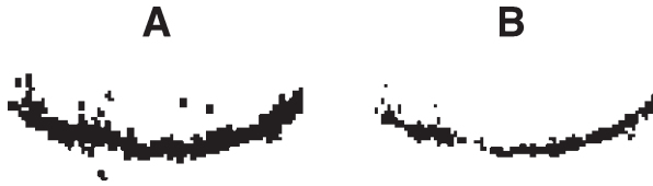
Fig. 8. Zoomed images comparing thresholded (peak) data to the full data set of a typical PM segment of DHE emission detected over the wavelength region 350–400 nm. (Panel A) Image before 75% thresholding was applied. (Panel B) Image after 75% thresholding was applied.
